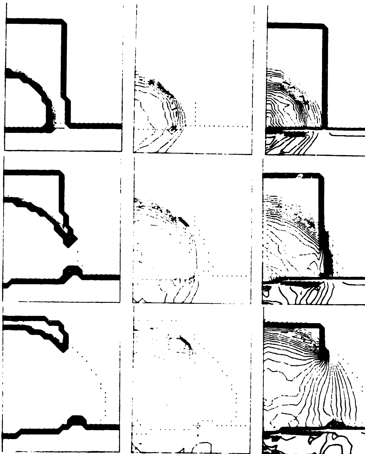
Fig. 8. Detonation of the donor cylinder (VRO-simulated 2-in. cube). Contour plots of mass fraction, pressure (40-kbar interval) and density (0.1 g/cm 3 interval).
